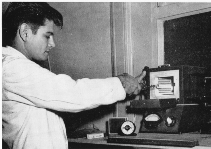
4) Heat treating, case hardening at 1200°F. by Emerson Smith
